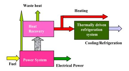
Figure 1. Schematic of a trigeneration system
