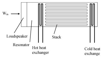
Figure 1 Sound wave Thermoacoustic engine
