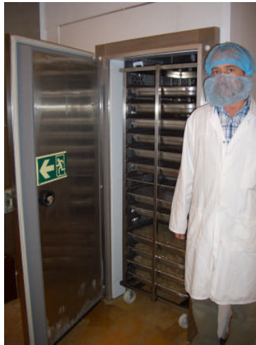
Figure 1: Pie-filling cooling room at Pieminister, (door dimensions – width = 71 cm, height = 174 cm ). Manufactured by Fosters
