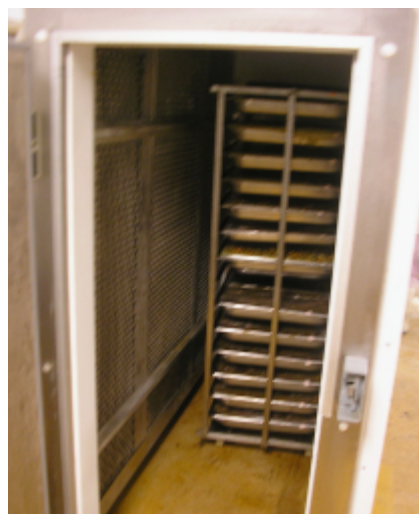
Figure 3. Example of push through blast chiller
