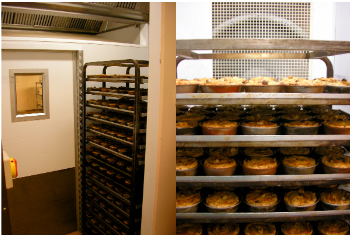
Figure 1. Two views of a trolley of hot pies being cooled in the ambient cooler prior to de-tinning
