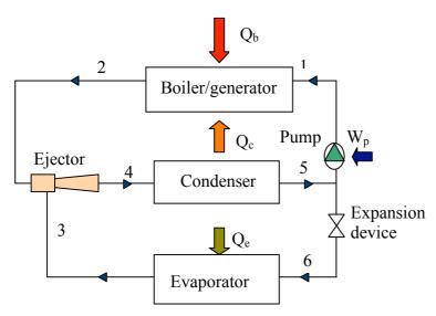
Referring to the basic ejector refrigeration cycle in Figure 1, the system consists of two loops, the power loop and the refrigeration loop. In the power loop, low-grade heat, Q<sub>b</sub>, is used in a boiler or generator to evaporate high pressure liquid refrigerant (process 1-2). The high pressure vapour generated, known the as primary fluid, flows through the ejector where it accelerates through nozzle. the The reduction in pressure that
