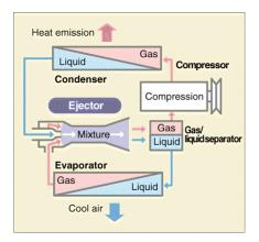
To improve the efficiency of the simple ejector cycle more complex cycles have been investigated [5] as well as the integration of ejectors with vapour compression and absorption systems. An example of this is the Denso transport refrigeration system [6]. Significant effort has also been devoted to the development of solar driven ejector refrigeration systems [7].
