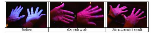
light indicates the user should rub the soap onto their hands. The light becomes solid on for the last 2 seconds of soaping indicating to the user that the rinse cycle is about to start. A 10 second high intensity rinse follows with the user moving their hands within the jets for maximum washing effectiveness. This prototype rig consistently removes UV gel from the whole hand and is as effective as a sink based wash of three times the duration.
