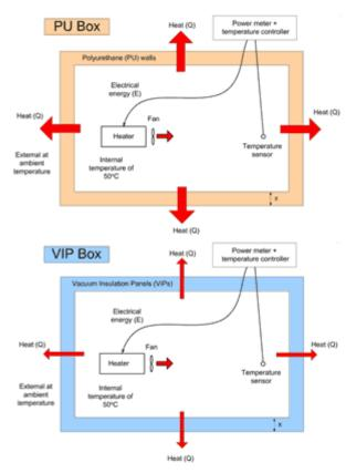
Vacuum insulating panels (VIPs) are a highly efficient insulation material that can be used for reducing the external size, increasing the internal size or increasing the thermal performance of many kinds of insulated containers and spaces.
